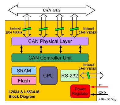
Figure 2-1 Block Diagram of the I-2534 & I-5534-M
