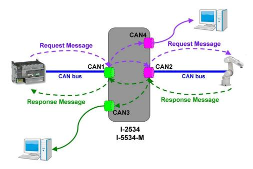
3. The route path needs to be configured as bellow CAN1 <--> CAN 2 and CAN 4 CAN2 <--> CAN 1 and CAN 3.
