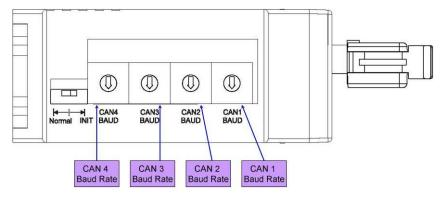
Figure 2-14 CAN baud rate configuration
