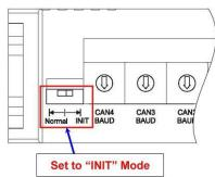
Figure 3-3 Set the I-2534 into the initial mode
