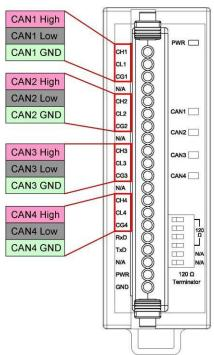
The figure 2-2 illustrates the CAN bus pins.
