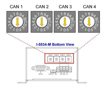
Figure 2-15 CAN baud rate configuration
