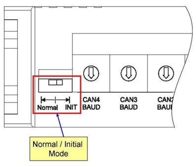
Figure 2-16 Operation Mode of the I-2534 module
