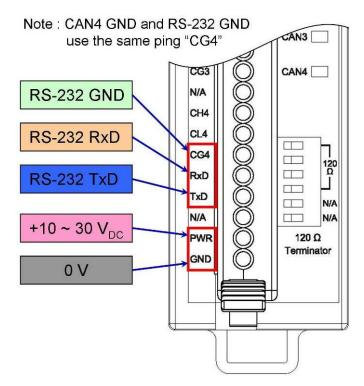
Figure 2-4 RS-232 and Power pin assignment of the I-2534
