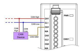
The CAN bus wire connection of the I-2534 is displayed in the figure 2-18.
