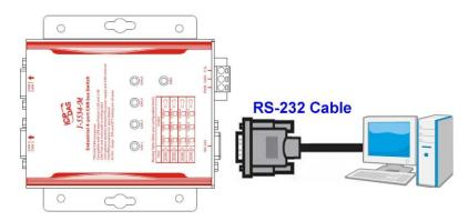
Figure 3-6 RS-232 wire connection of the I-5534-M
