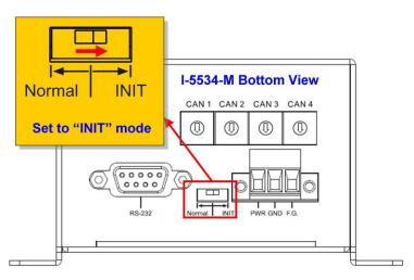
Figure 3-4 Set the I-5534-M into the initial mode
