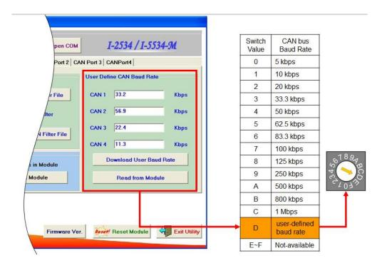
Figure 3-10 CAN user-defined baud rate configuration
