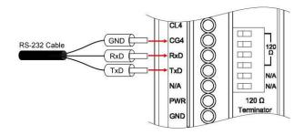
Figure 3-5 RS-232 wire connection of the I-2534
