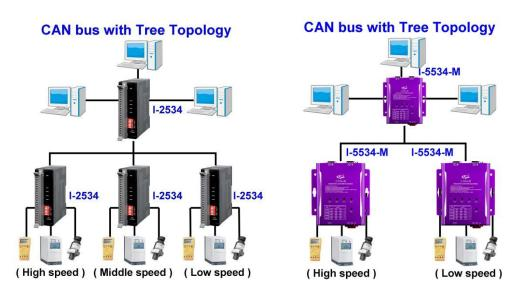
Figure 3-2 Tree topology with the I-2534 and I-5534-M
