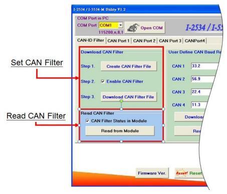
Figure 3-11 Set and read the CAN filter configuration
