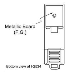
Figure 2-19 Metallic Board at Back of the I-2534
