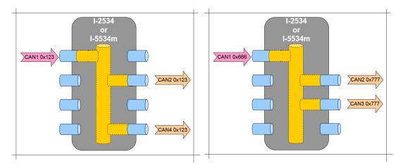
Figure 3-28 CAN1 dependent CAN-ID routing rule
