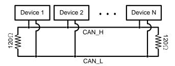
Figure 2-11 120Ω terminal resistor position
