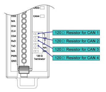
Figure 2-8 120 $\Omega$  terminal resistors of the I-2534
