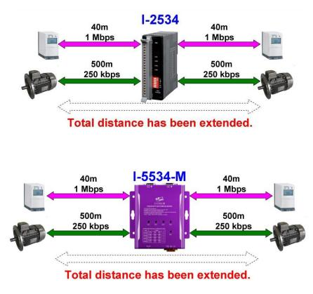
Figure 1-1: Application to extern the transmission distance
