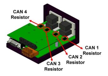
Figure 2-9 120 $\Omega$  terminal resistors of the I-5534-M
