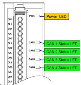
The figure 2-6 shows the names and statuses of the LEDs.
