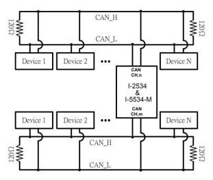
Figure 2-13 Disable the 120Ω terminal resistors of the I-2534 / I-5534-M
