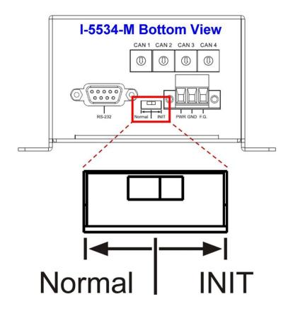
Figure 2-17 Operation Mode of the I-5534-M module
